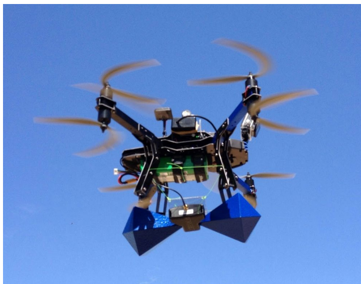
The External Calibrator for Hydrogen Observatories (ECHO) configuration at the time of the August 2015 testing. A broadband bowtie dipole is slung beneath an octoquad UAV (an X8+ from 3DR).
