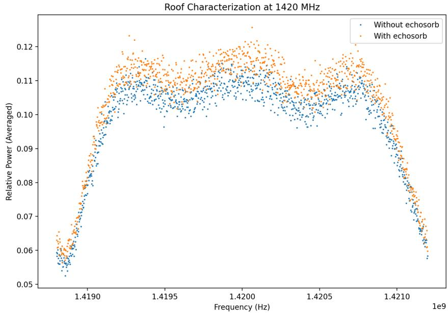
Figure 18. Average of 400 integrations centered at 1420 MHz, with and without the echosorb on the horn.
