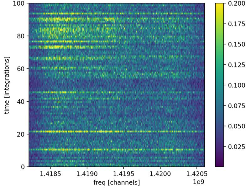
Figure 17. 100 integrations at a center frequency of 1419.405752 MHz, 1 MHz from the 21cm line.
