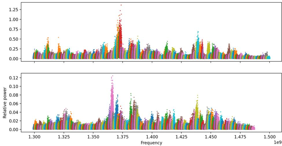
Figure 16. Comparison of two scans. The top scan was shown in previous figures, as a single integration from 1300-1500 MHz with no averaging. The bottom scan is a single integration from 1300-1486 MHz, averaged over 10 tunings.
