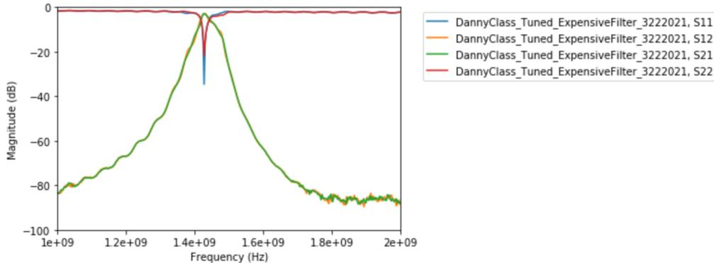
Figure 12. Commercial filter from K&L tuned for the 21cm line using a cavity resonator design
