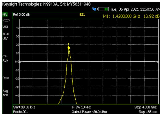
Figure 10. Gain of ZX60 LNA + KL Filter setup at 1.42 GHz
