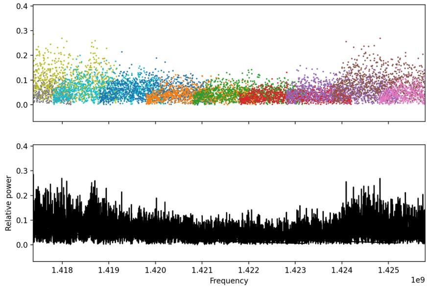
Figure 15. Single integration from 1300-1500 MHz with no averaging, pointed directly up at the sky, zoomed in at 1420 MHz.
