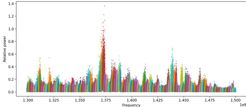
Figure 14. Single integration from 1300-1500 MHz with no averaging, pointed directly up at the sky.
