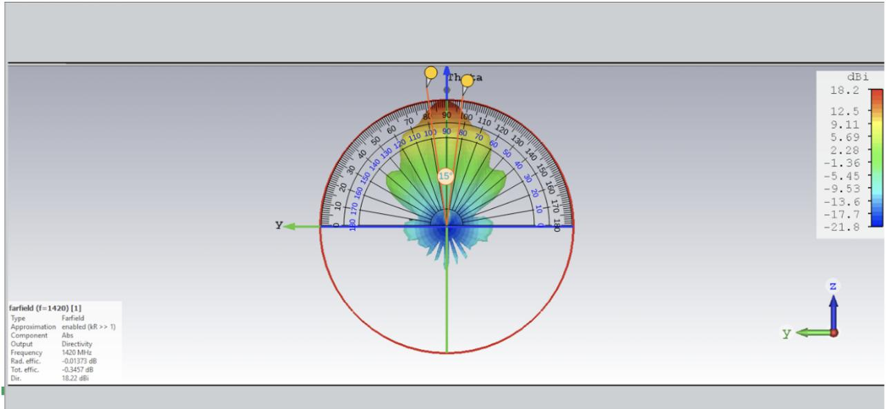
Figure 2.  $\theta_{beam}$  calculations from beam pattern simulations using an online protractor
