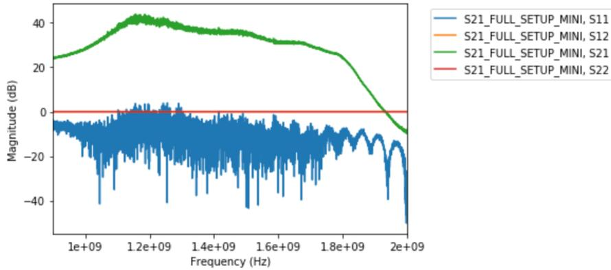
Figure 11. Mini-Circuits filter for around the 21cm line, including 2 amplifiers in the chain.
