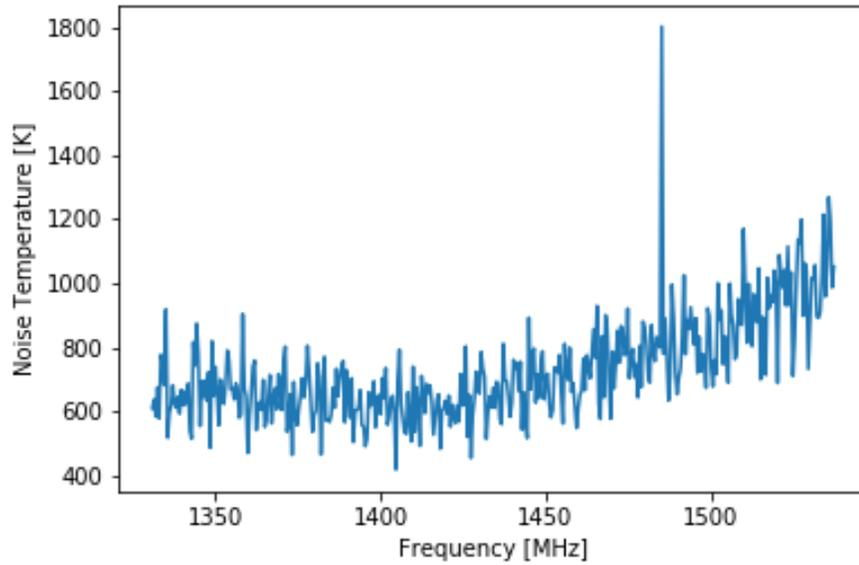
Figure 7. Noise temperature as a function of frequency for the cascaded chain of two budget amplifiers.
