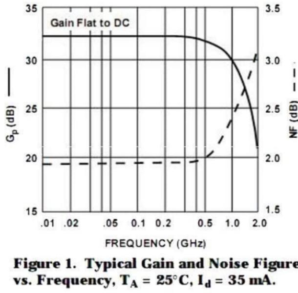
Figure 6. Budget amplifier noise and gain as a function of frequency.
