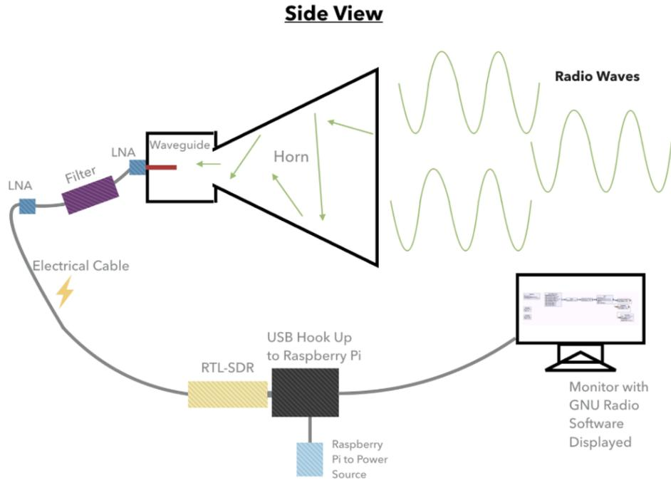
Figure 4. A schematic diagram of the measurement setup
