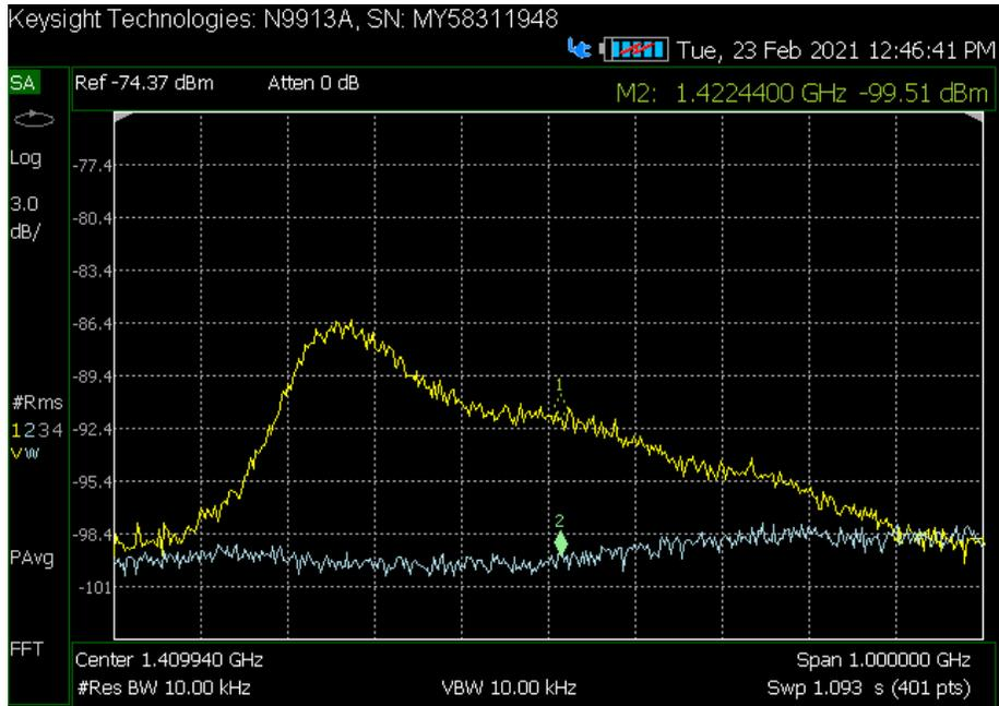
Figure 9. Noise introduced by the Budget LNAs
