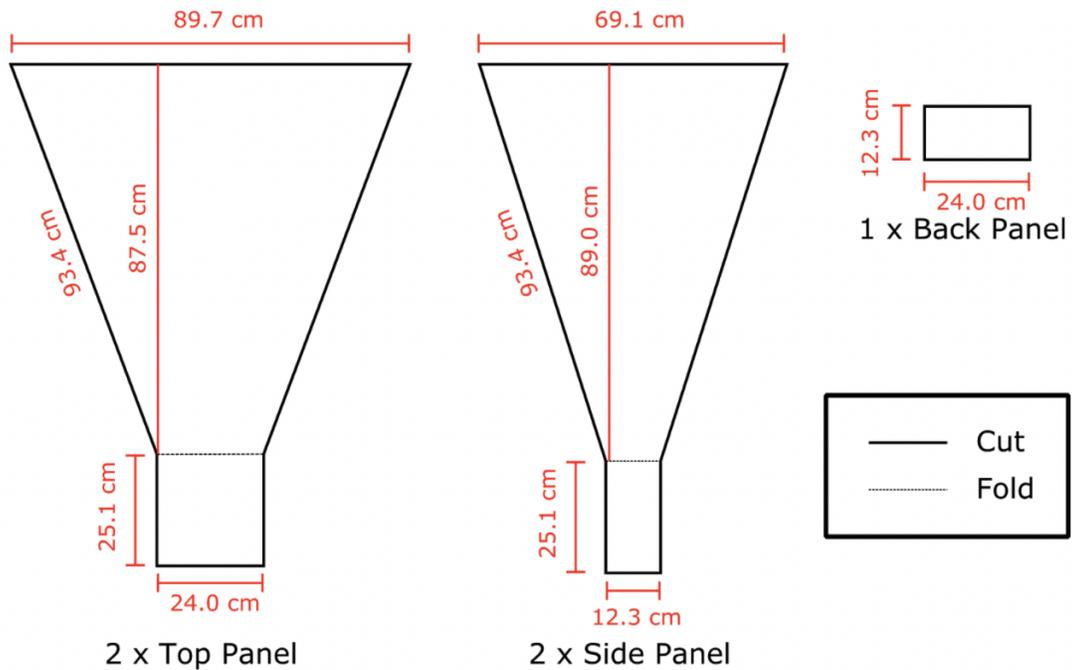
Figure 5. Dimensions of the horn antenna
