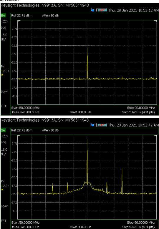
Spectrum from 50MHz to 90MHz with a 300Hz bandwidth. Off peak is about -25dB and On peak is about +15dB, meaning the switch is able to isolate about 40dB in this setup. There is possibly some compression due to overloading the Fieldfox.
