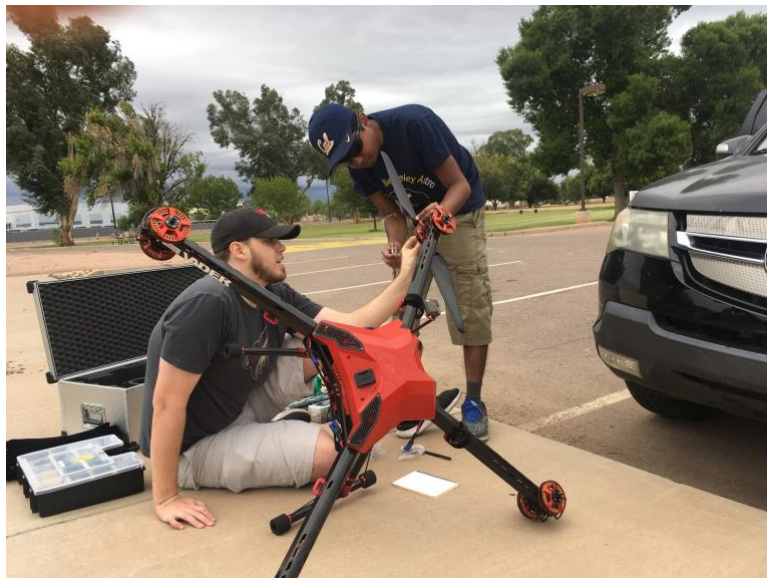
Figure 3: The Steadidrone Vader met all requirements for mounting, flight time, and stability. But ultimately was not used because of repairability and safety.
