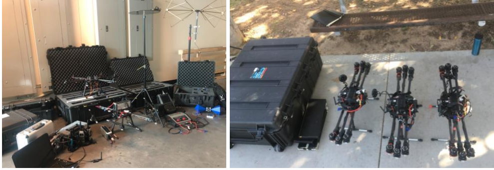
Figure 1: The ECHO-2 external calibration kit emphasizes redundancy with multiple drones (currently three), an independent spectrum monitor (collapsible bicone for <100MHz operation + Fieldfox spectrum analyzer), batteries chargers, independent ground station computer.
