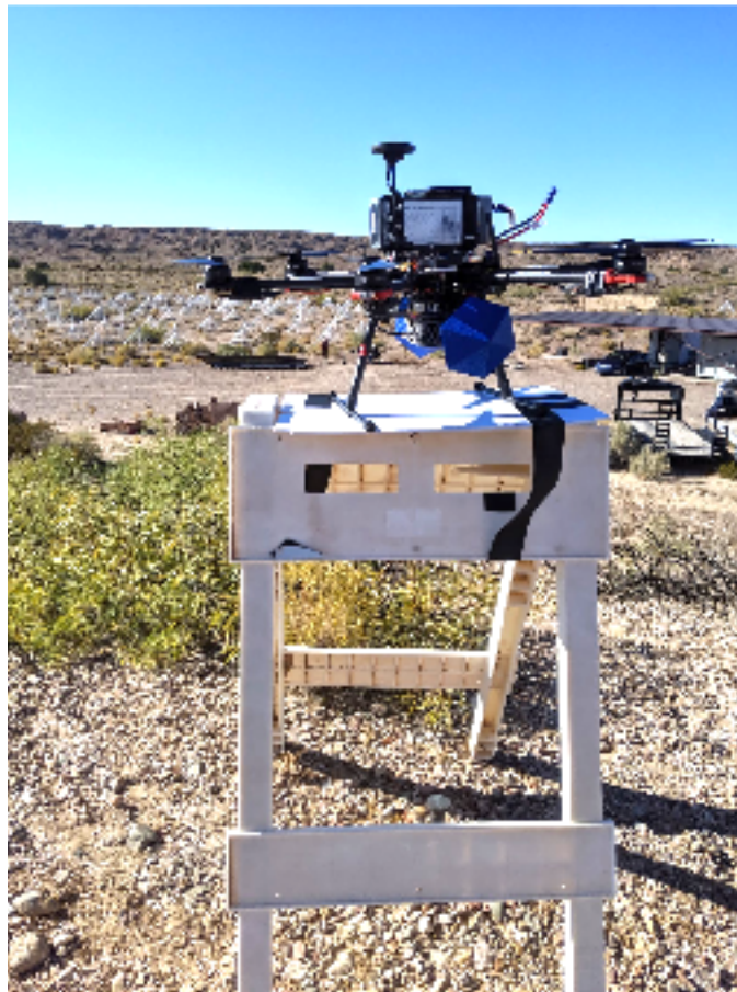
Fig 1: Experimental setup for the phase experiment. The ECHO drone is placed above the survey marker.
