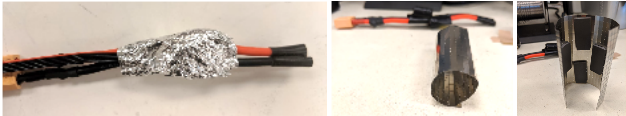
Fig 5: Different shielding methods. From Left: tinfoil, bendable metal enclosure, bendable enclosure with absorbers
